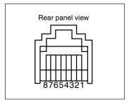
**CAUTION: DO NOT** short pin 1 to ground as this can damage the internal 8 V regulator.
